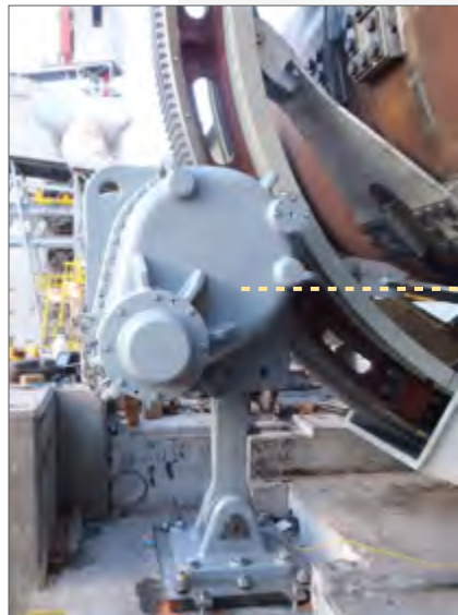
Bogiflex KGD self-aligning kiln gear drive
