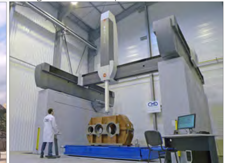
3D measuring machine for large-size XXL workpieces
