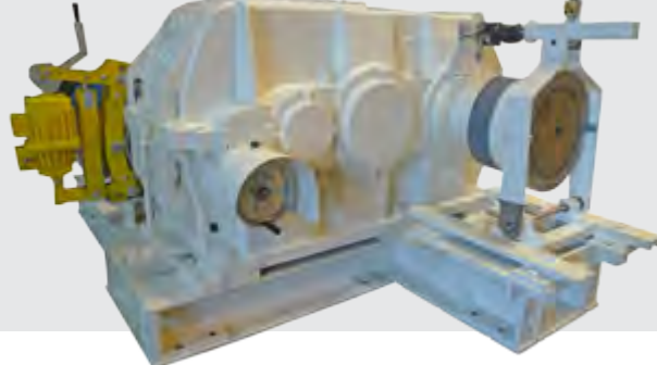
ERmaster Inching drive brake system
