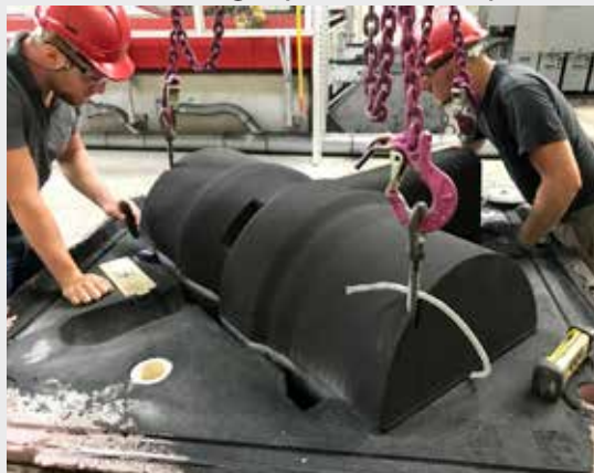
5 - Machined sand cores moulding operation set up
