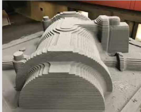
2 - Sand block rough milling operation
