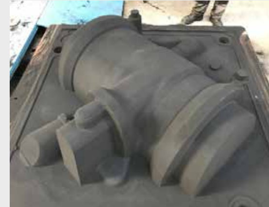
3 - Sand block final milling operation
