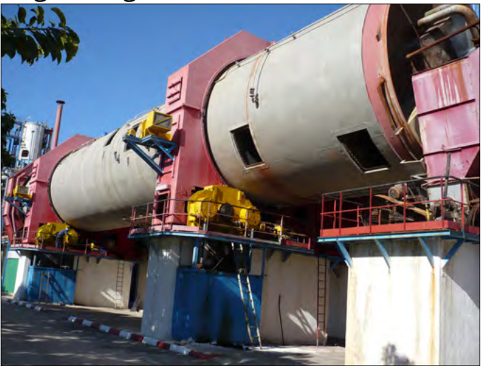
Bogiflex® gearbox for horizontal diffuser drive or dryers
