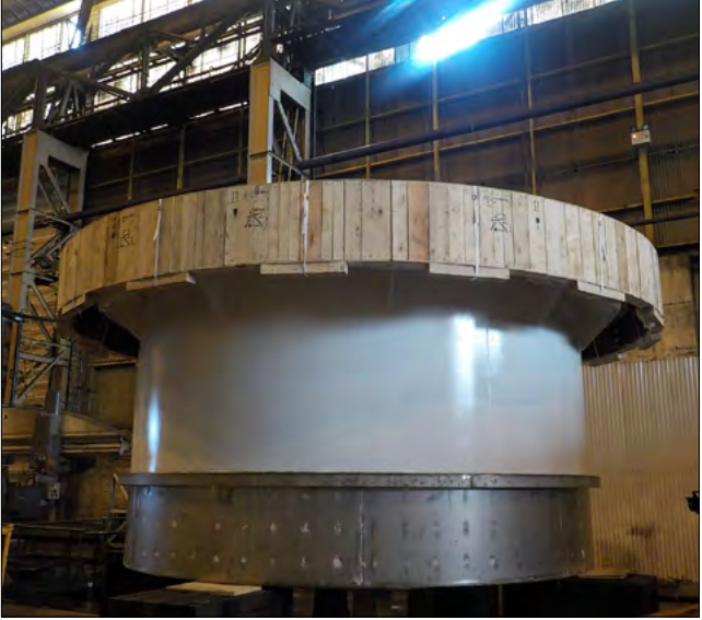
Vertical diffuser upper part shell
