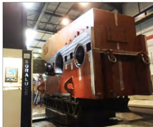
Machining of casing on CNC boring machine
